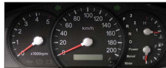
Large size speedometer, LCD odometer and tripmeter
